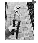
Find a tool that will do the job. Decide on a place it will ALWAYS BE. Write it on "House Stuff." The closer the location of the shut-off tool to the gas meter, the better. You could even zip-tie the tool to your meter so it's always there. Make sure to make it loose enough to be able to angle it for use, or you will need a pair of scissors to cut it off before using it! If you do not have one, write it on your "Things Needed" list.
